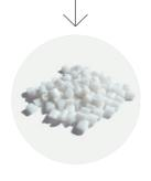
These flakes are melted into chips and blown into polyester staple fibre.
